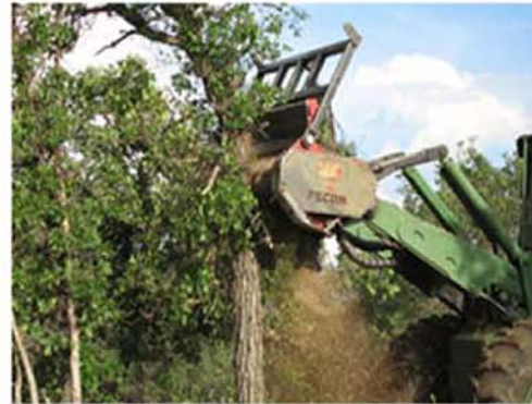
A loader-type, rubber-tired platform reaches out with its specially designed head and removes the top of the tree.
